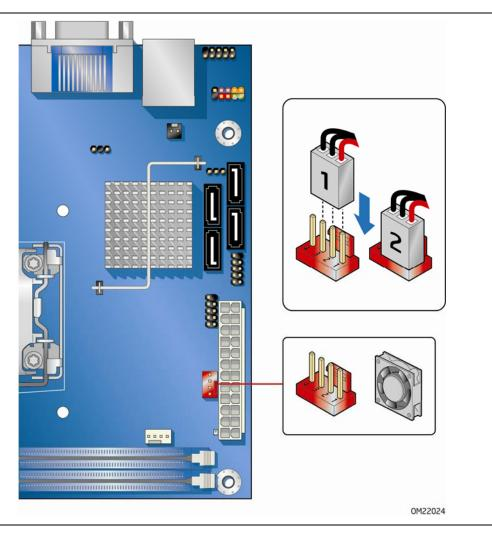
Figure 22. Location of the Chassis Fan Header
